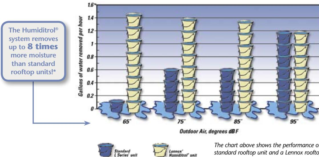
The chart above shows the performance of a standard rooftop unit and a Lennox rooftop unit with Humiditrol® dehumidification option.
